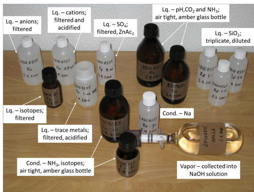
FIGURE 2: Sample aliquots collected during single sampling of two-phase well. Liquid (Lq.), condensate (Cond.), and vapour sample are taken into appropriate containers and preserved for further analysis according to Table 1.
