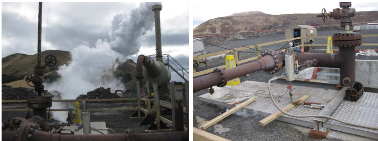
FIGURE 1: Sampling of the two-phase well during the discharge test. The well head is connected to a transportable steam separator which discharges steam into the air and water into a weir box where fluid flow is quantified (e.g. Axelsson, 2018).
