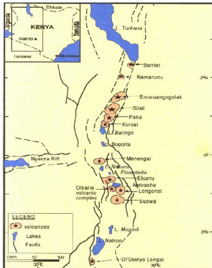
FIGURE 9: Apex of Kenya Rift domal uplift with two volcanically active rift branches and a third E-W branch dying. Stratovolcanoes are shown. Fissure swarms have not been identified as integral parts of volcanic systems (Mwawongo 2004)
