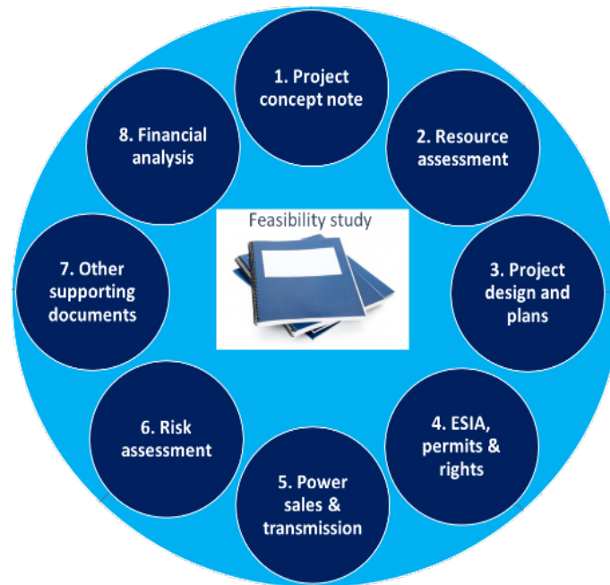
FIGURE 6: An overview of a business case or set of bankable documents, where at the centre is the feasibility study
