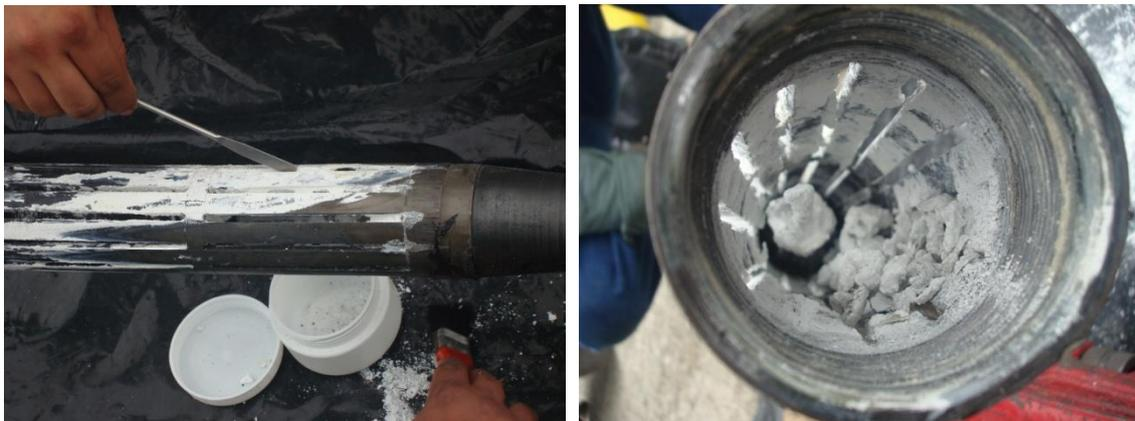
FIGURE 4: Inhibitor's solid by-products deposited in the injection system.
