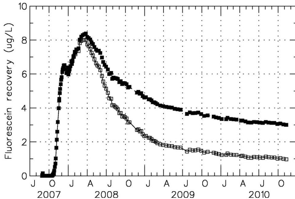
FIGURE 9: Fluorescein recovery in production well HO-1 in the Hofstadir low-temperature system in W-Iceland (see Figures 3 and 7), following the injection of 10 kg of the tracer into reinjection well HO-2 (from Axelsson, 2011). The test lasted 3.5 years. The lower curve shows the recovery corrected for the tracer being reinjected (recirculated) after production from HO-1. About 70% of the tracer was recovered during the test
