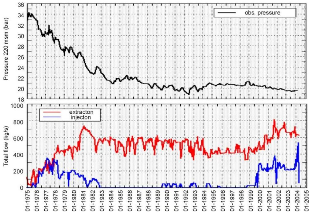
FIGURE 5: The production, reinjection and pressure response history of the Ahuachapan geothermal system in El Salvador (see also Monterrosa and Montalvo, 2010)
