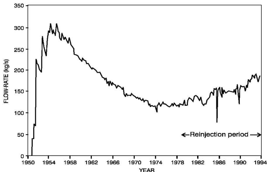
FIGURE 1: Flow-rate history of wells in the Larderello – Valle Secolo area, Italy, since the early 1950's demonstrating the benefit of reinjection (from Capetti et al., 1995)
