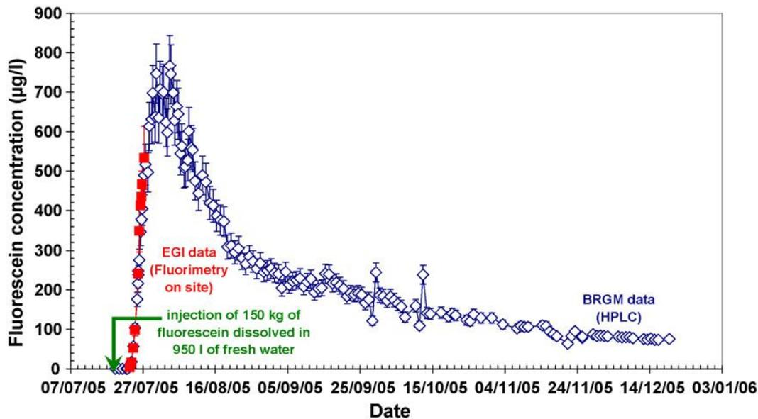
FIGURE 11: Fluorescein recovery in well GPK-2 at the Soultz EGS-site in N-France, following the injection of 150 kg of fluorescein into well GPK-3 (figure from Sanjuan et al., 2006). The test lasted 5 months. About 24% of the tracer was recovered during the test
