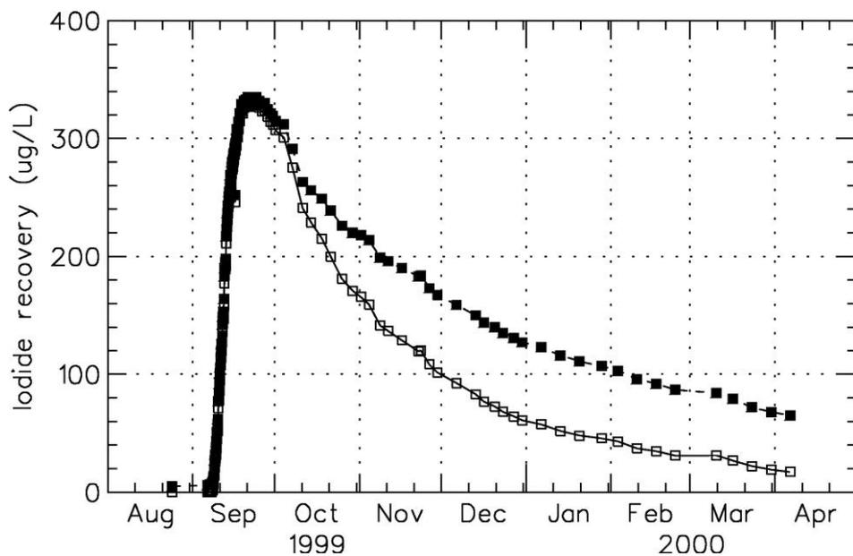
FIGURE 10: Iodide recovery in production well K-21 in the Krafla high-temperature system in N-Iceland, following the injection of 200 kg of KI into well K-22 (from Axelsson, 2011). The test lasted 7 months. The lower curve shows the recovery corrected for the tracer being reinjected (recirculated) after production. About 30% of the tracer was recovered during the test)
