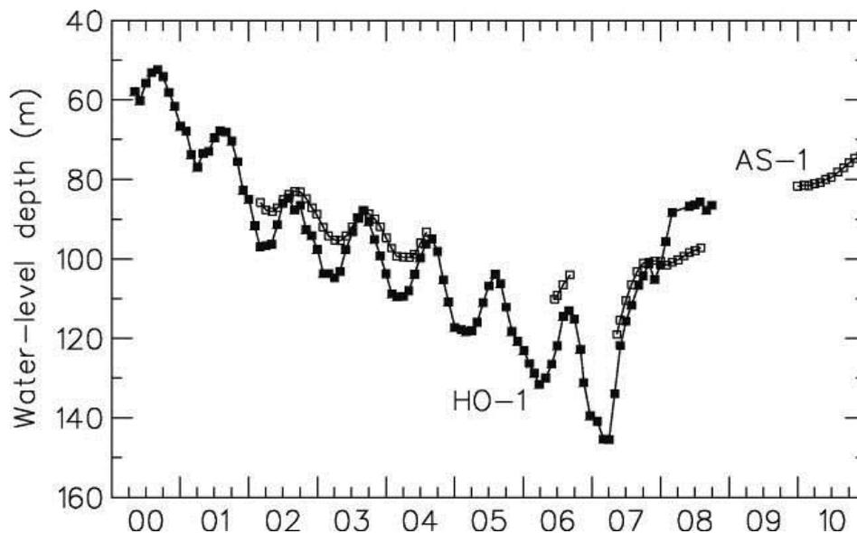
FIGURE 7: Pressure changes in the Hofstadir low-temperature geothermal system in W-Iceland during the first 11 years of production, shown as water-level changes in the main production well (HO-1) and in a monitoring well (AS-1). A continuous pressure decline for 7 years is reversed in the spring of 2007 when reinjection commences. Figure from Axelsson (2011)
