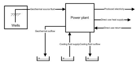
FIGURE 1: Schematic of a geothermal power plant
