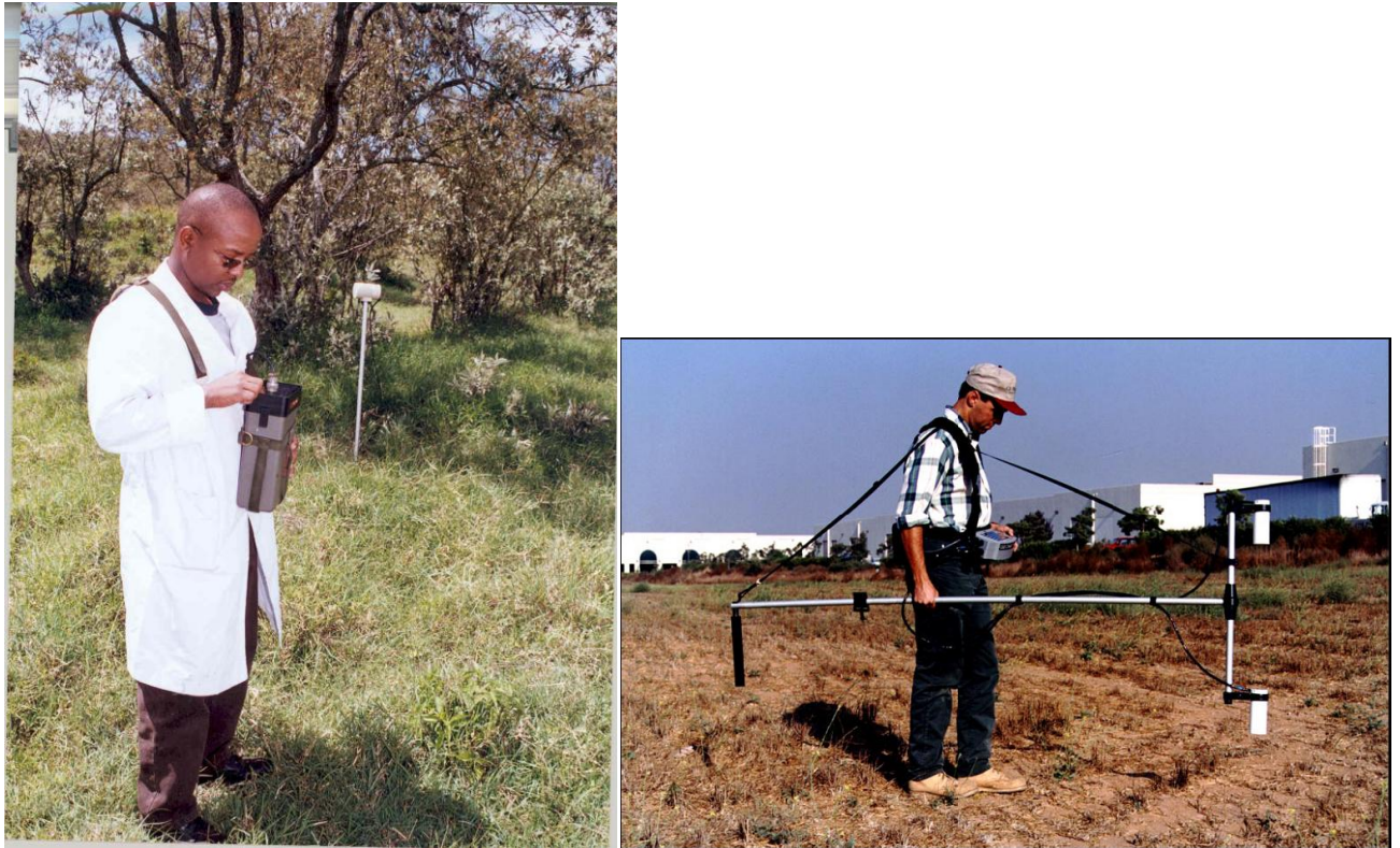
FIGURE 1: Proton Precession magnetometers. (a) Geometrics G-856 (b) Geometrics G-858
