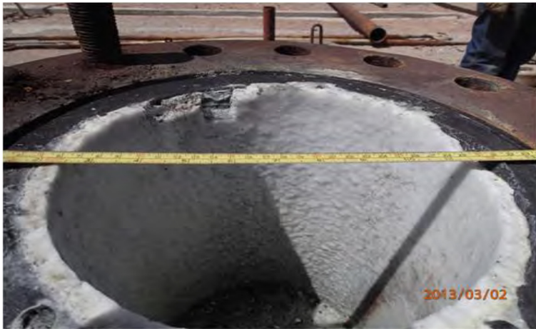
FIGURE 10: Well SM-5, teschemacherite coats the well (JICA 2013; Villarroel, 2014)
