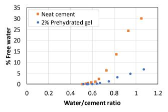
FIGURE 11: Effect of water/cement ratio on the free water in class A cement (neat) and class A cement with 2% bentonite
