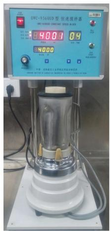
FIGURE 2: Vane type sample mixer used by GDC
