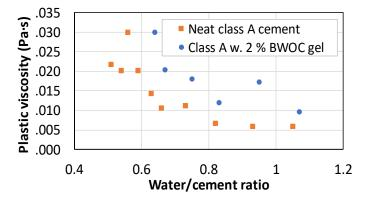
FIGURE 13: Effect of water/cement ratio on plastic viscosity in class A cement (neat) and class A cement with 2% bentonite
