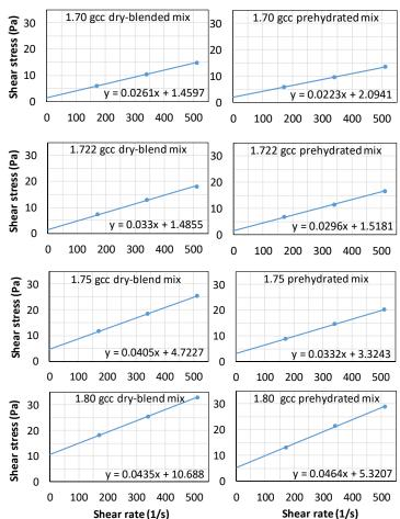
FIGURE 16: Shear stress/shear rate plots for dry-blended and pre-hydrated slurries
