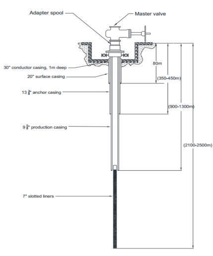
FIGURE 6: Well design for Menengai geothermal wells
