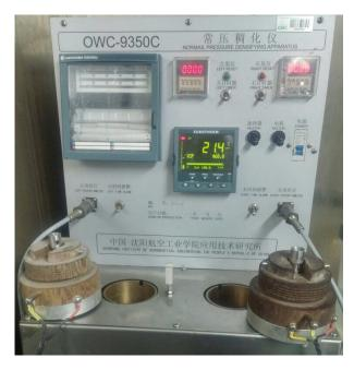
FIGURE 4: Atmospheric consistometer used by GDC
