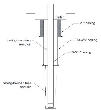
FIGURE 8: Production casing cementing
