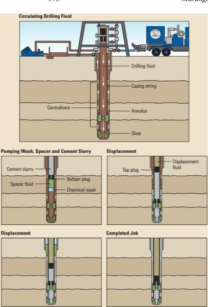
FIGURE 7: Single stage cementing process (Nelson, 2012)
