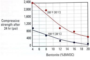
FIGURE 15: Effect of bentonite on compressive strength (Nelson and Guillot, 2006)
