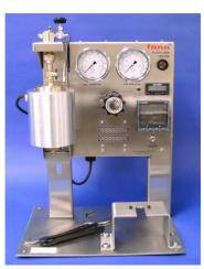
FIGURE 3: Fluid loss cell (Fann, 2014)
