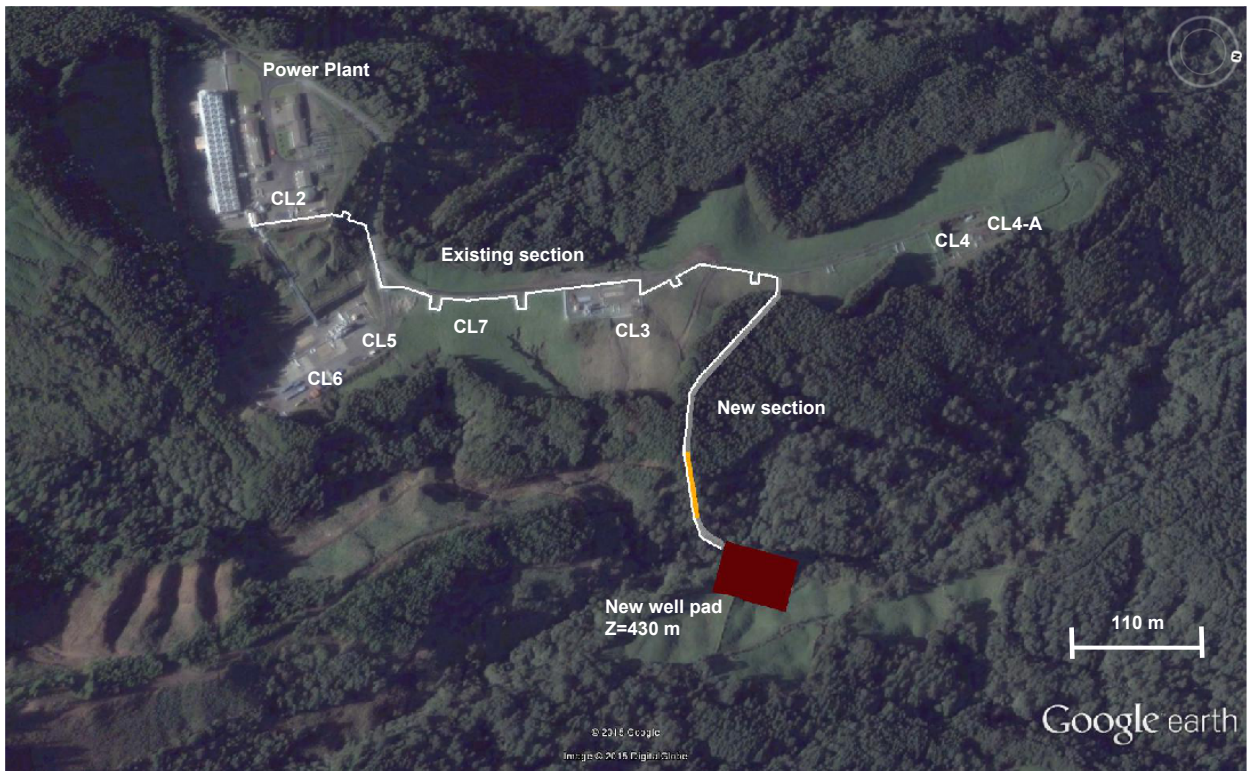
FIGURE 1: Gathering system pipe route from well pad to the plant (Google Earth)
