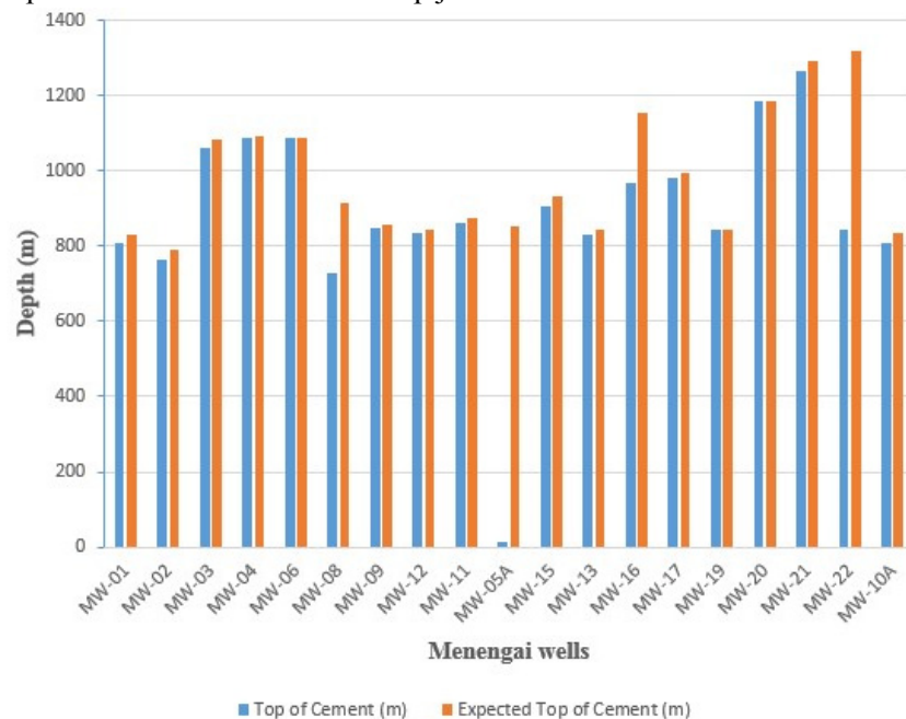
FIGURE 12: Graph showing comparison of actual top of cement and expected top of cement depths inside the production casing
