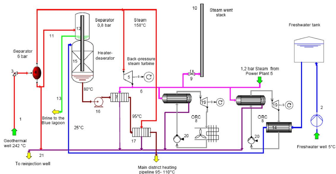
FIGURE 7: Flow diagram of Svartsengi power plant (Thorolfsson, 2005b)
