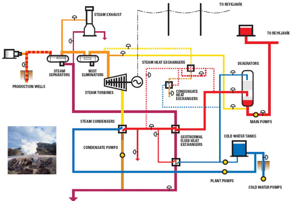
FIGURE 8: A Flow diagram of Nesjavellir geothermal power plant (Reykjavik Energy, 2003)
