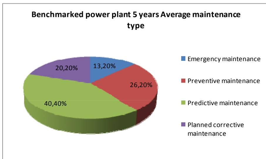
FIGURE 9: Five years' average maintenance types used by the benchmarked power plant
