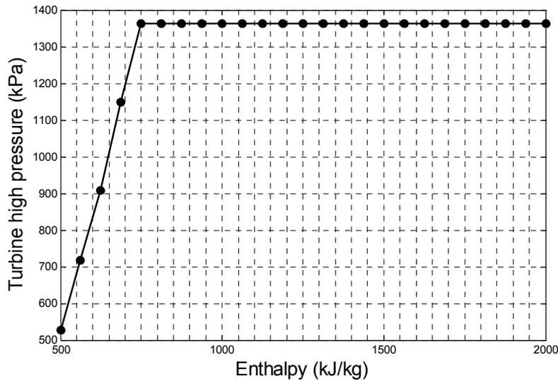
FIGURE 31: High turbine pressure vs. enthalpy
