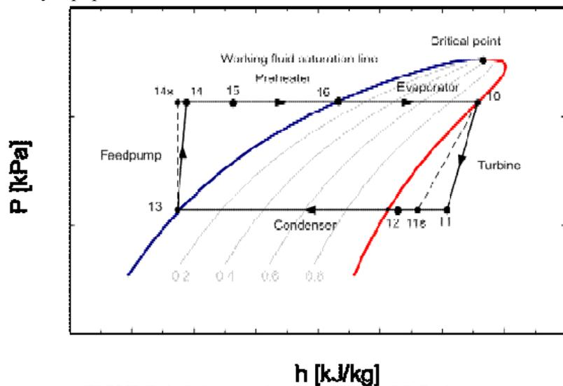
FIGURE 6: P-h state diagram for an ORC plant
