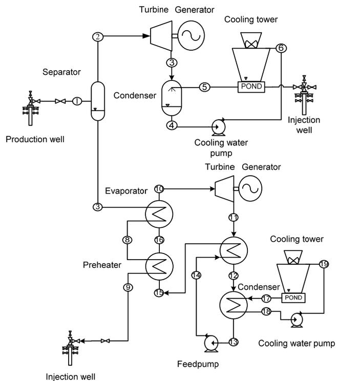
FIGURE 5: Simplified schematic diagram of a combined single and ORC plant
