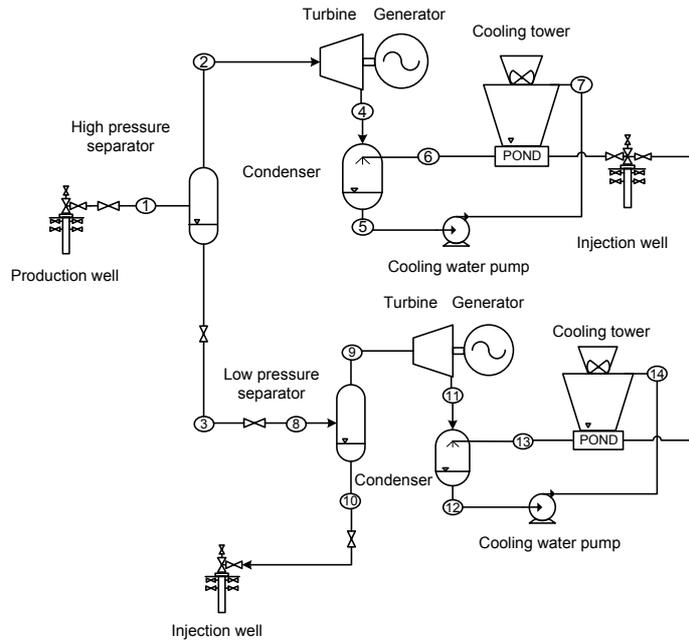
FIGURE 3: Simplified schematic diagram of a combined single and second flash plant
