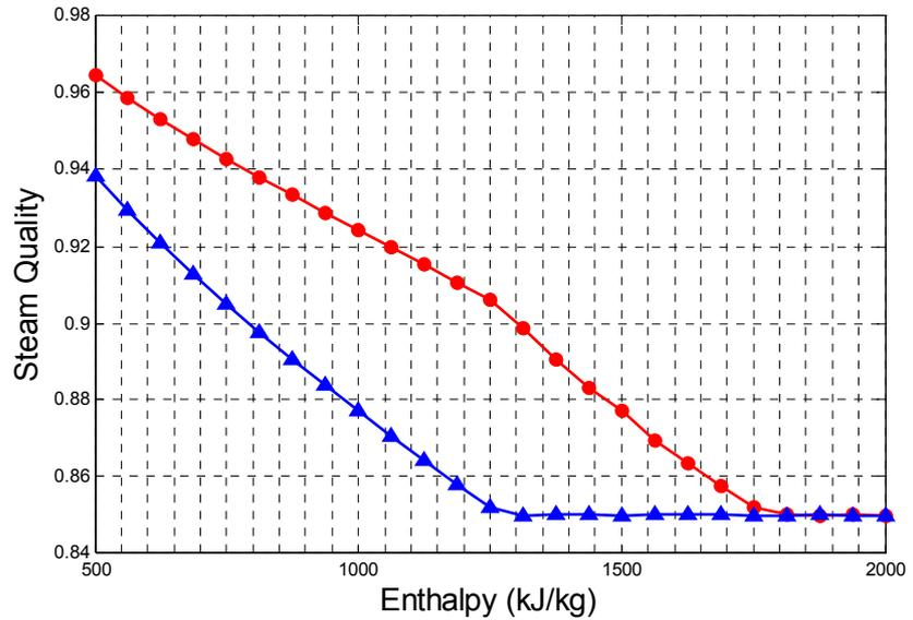
FIGURE 16: Double flash turbine exhaust steam quality vs. enthalpy
