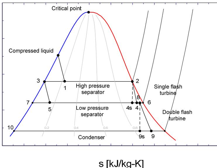
FIGURE 2: T-s state diagram for a double flash plant
