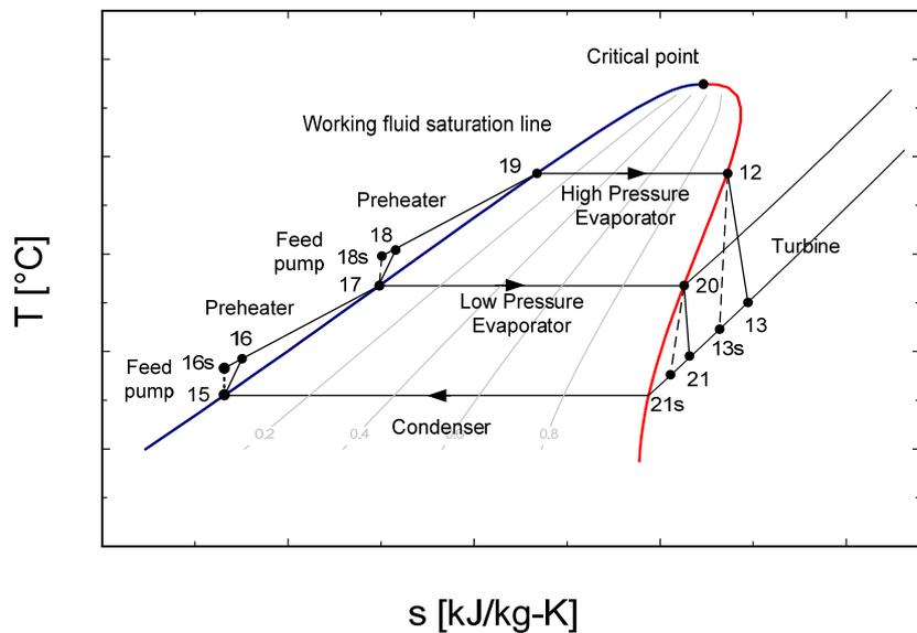
FIGURE 10: T-s state diagram for an advanced ORC plant
