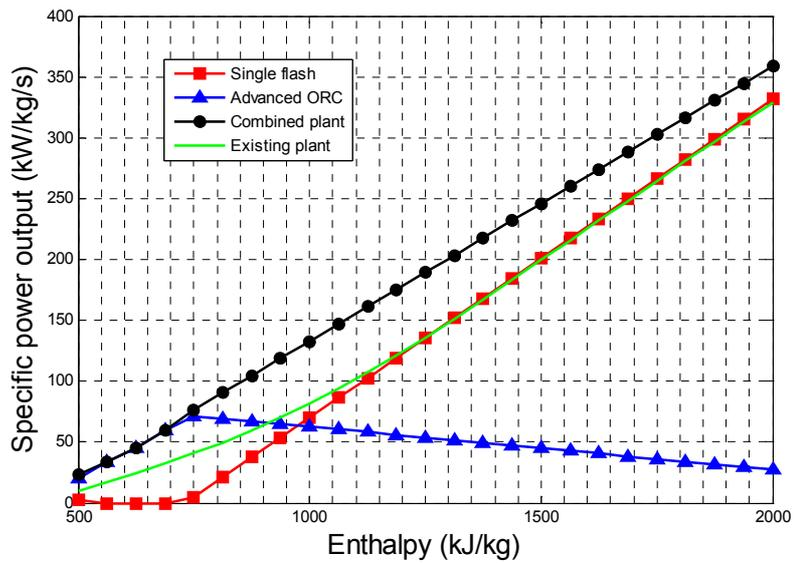
FIGURE 28: Specific power output of a combined single flash and advanced ORC vs. enthalpy
