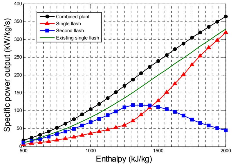
FIGURE 13: Specific power output of the double flash plant vs. enthalpy
