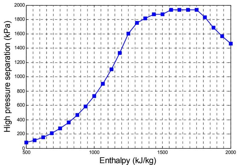
FIGURE 14: High pressure separation of the double flash plant vs. enthalpy
