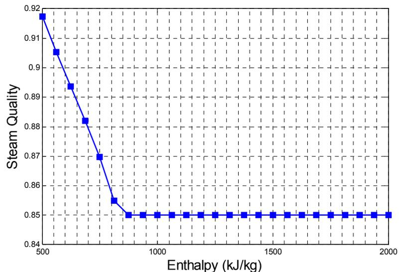
FIGURE 25: Single flash turbine exhaust steam quality vs. enthalpy
