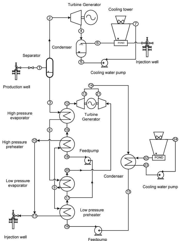
FIGURE 8: Simplified schematic of a combined single flash and advanced ORC plant
