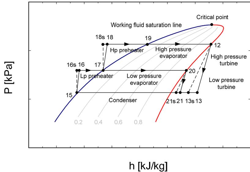
FIGURE 9: P-h state diagram for an advanced ORC plant
