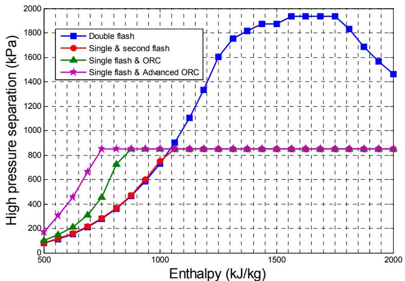
FIGURE 37: Comparison of separation pressures of different combined plants vs. enthalpy power generation
