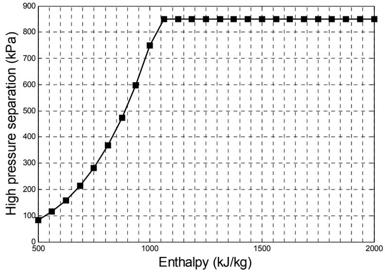
FIGURE 19: High pressure separation of a combined single and second flash plant vs. enthalpy
