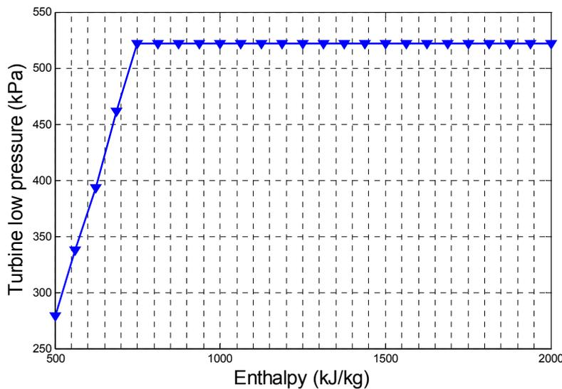
FIGURE 32: Low turbine pressure vs. enthalpy
