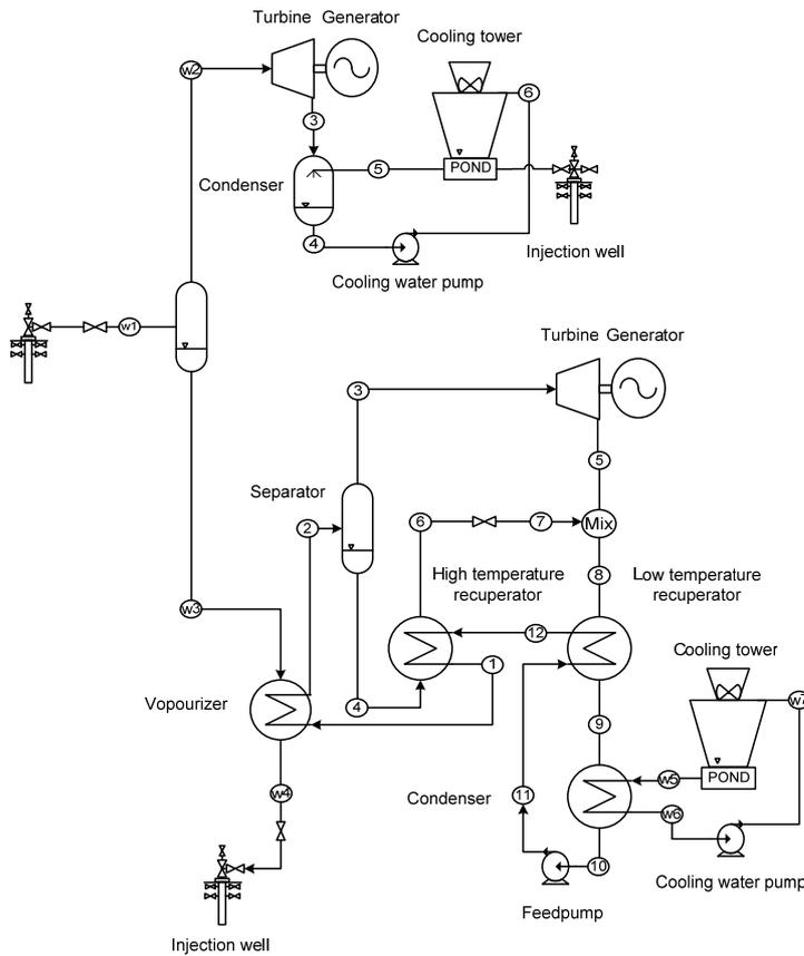
FIGURE 11: Simplified schematic diagram of a combined single flash and Kalina cycle plant
