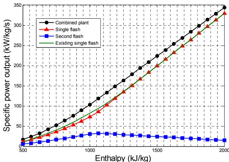
FIGURE 18: Specific power output of the combined single and second flash plant vs. enthalpy
