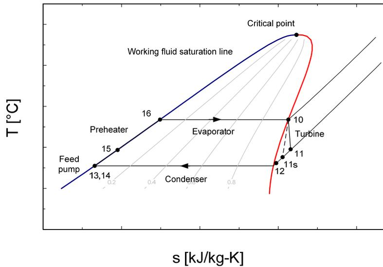
FIGURE 7: T-s state diagram for an ORC plant
