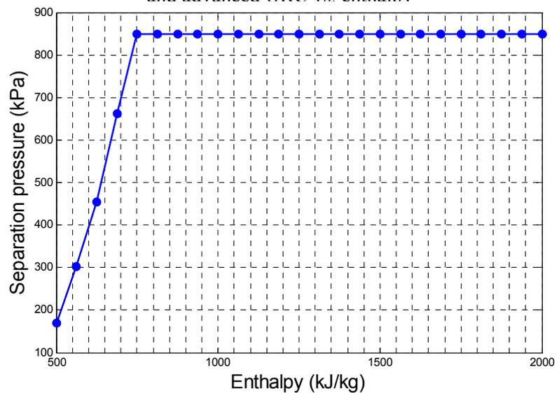
FIGURE 29: Separation pressure of a combined single flash and advanced ORC vs. enthalpy
