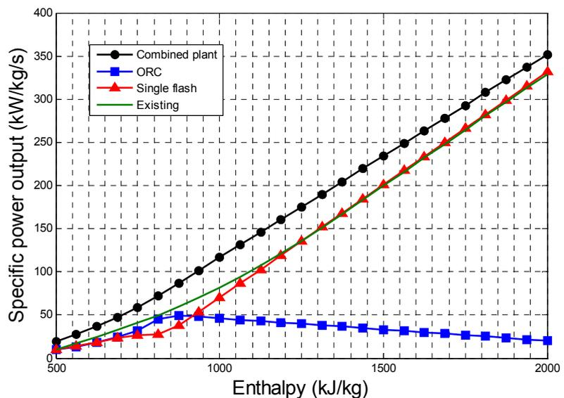
FIGURE 23: Specific power output of a combined single flash and ORC vs. enthalpy
