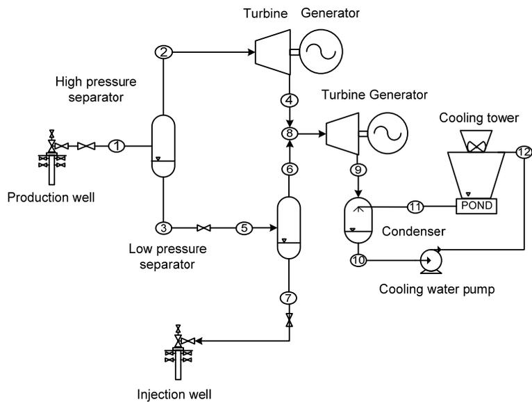
FIGURE 1: Simplified schematic diagram of a double flash plant
