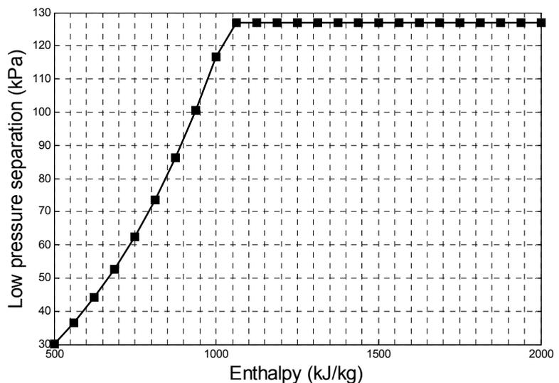
FIGURE 20: Low pressure separation of a combined single and second flash plant vs. enthalpy
