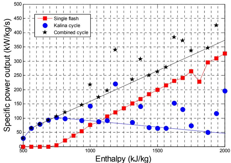
FIGURE 34: Specific power output of a combined single flash and Kalina cycle vs. enthalpy
