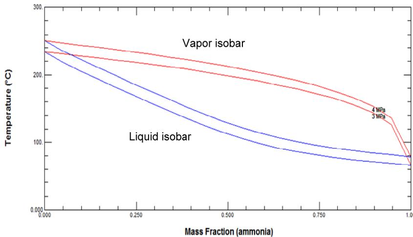
FIGURE 12: T-x diagram of ammonia-water
