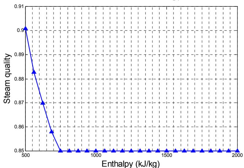
FIGURE 30: Steam quality of the single flash turbine exhaust vs. enthalpy
