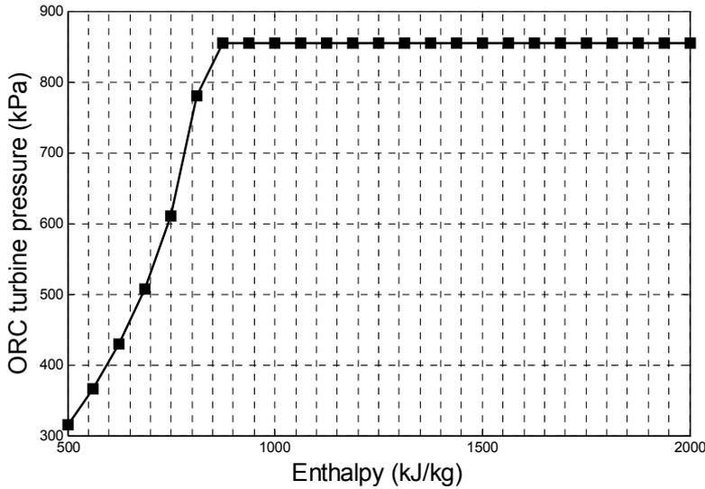
FIGURE 26: ORC turbine pressure vs. enthalpy
