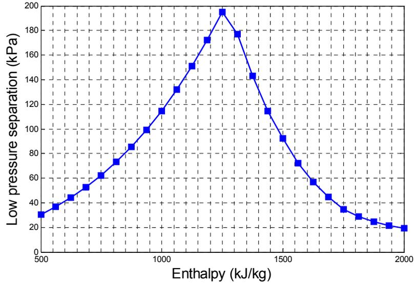
FIGURE 15: Low pressure separation of the double flash plant vs. enthalpy
