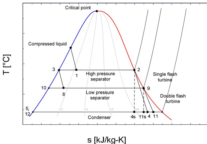
FIGURE 4: T-s state diagram for a combined single and second flash plant
