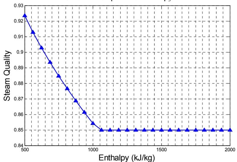
FIGURE 21: Single and second flash turbine exhaust steam quality vs. enthalpy
