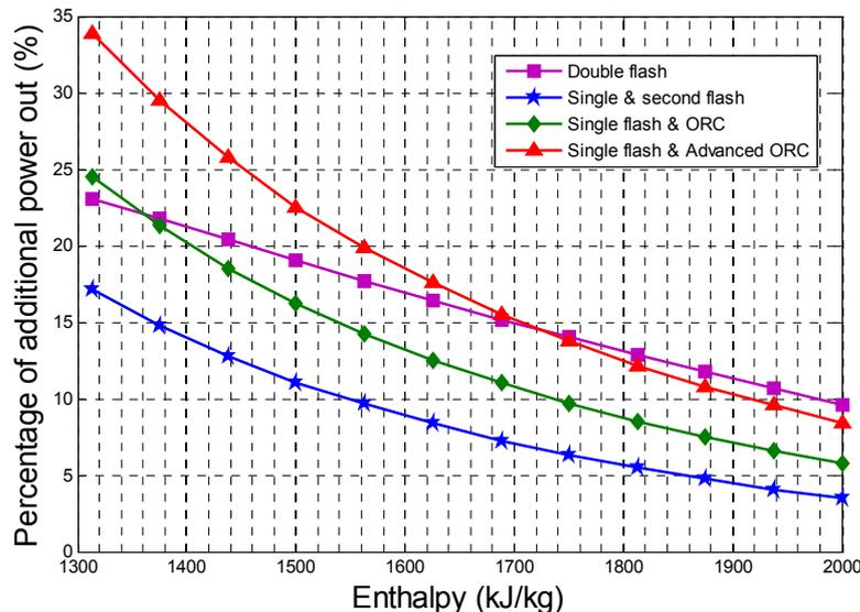
FIGURE 36: The percentage of additional specific power output of combined plants vs. enthalpy kJ/kg, the double flash plant gave the highest additional specific power output.
