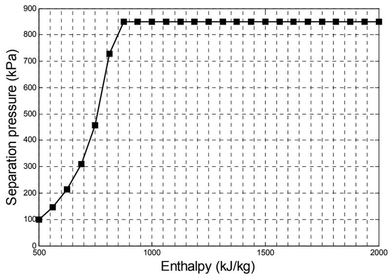
FIGURE 24: Separation pressure of a combined single flash and ORC vs. enthalpy
