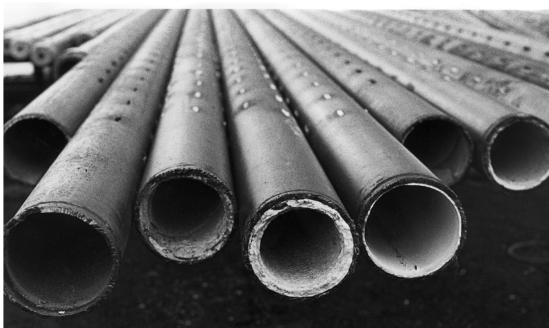
Figure 10: Calcite scaling inside a liner. Note that some slots are plugged.
