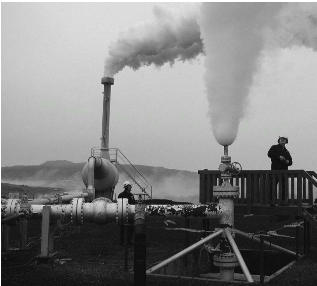
Figure 6: Starting a well to flow by opening a 3" valve on the wellhead to release the compressed air. Once steam comes to surface the flow is diverted to the separator/silencer.
