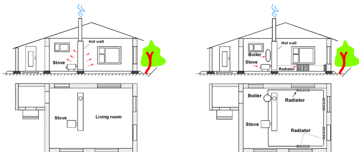
FIGURE 12: Individual house heating scheme
