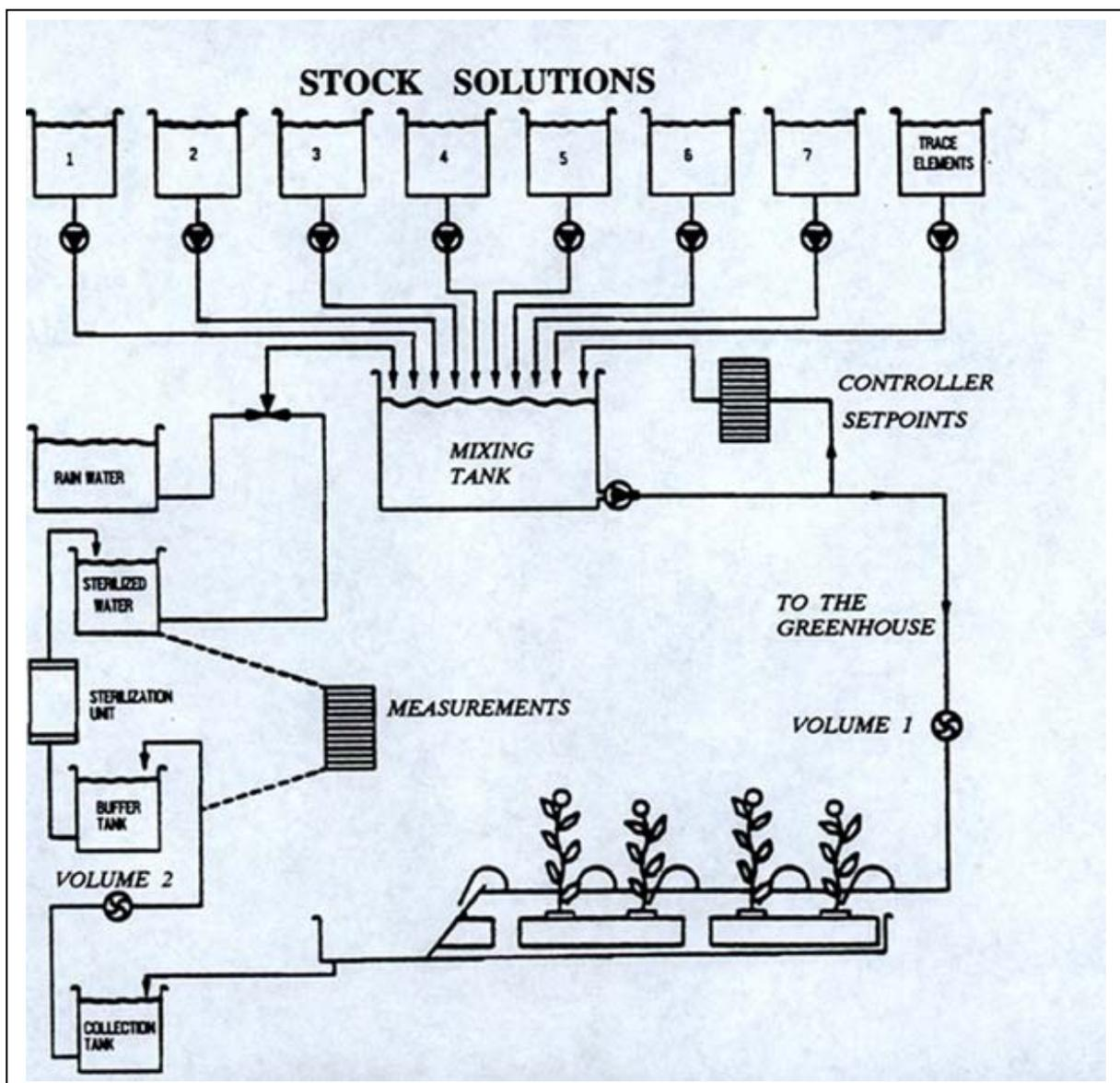
FIGURE 4: Closed-loop nutrient control system (Hanan, 1998)
