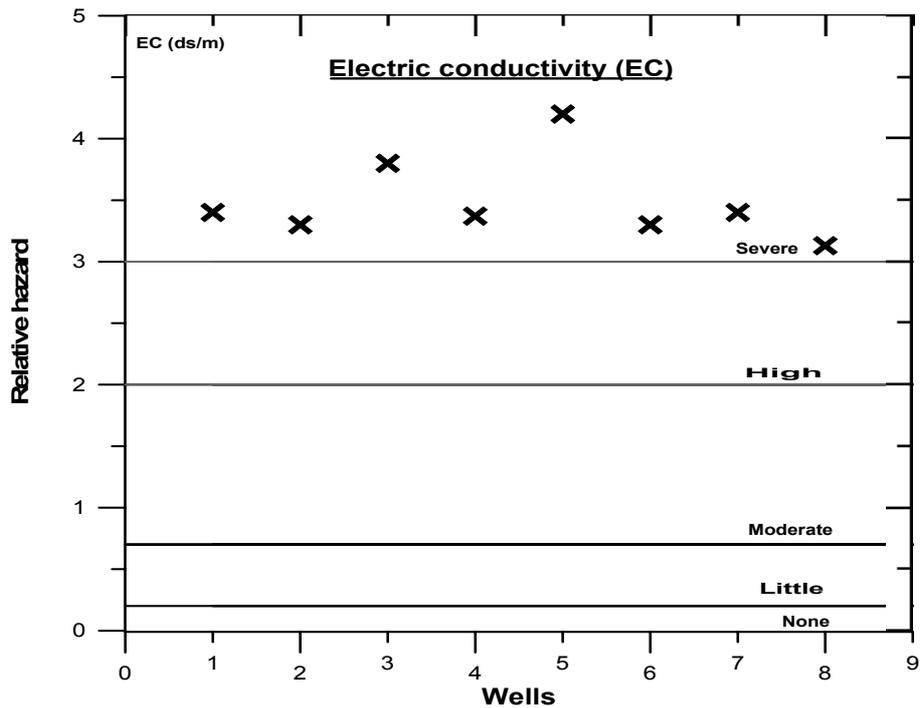
FIGURE 5: Relative hazard due to electric conductivity (EC) in the 8 chosen wells; the axis is numbered from 1 to 8, where 1 is Steftimi, 2 is Kebili, 3 is Om-elfarth, 4 is Limaguess, 5 is Jemna, 6 is Bouebdellah, 7 is Om-somaa and 8 is Debebcha.
