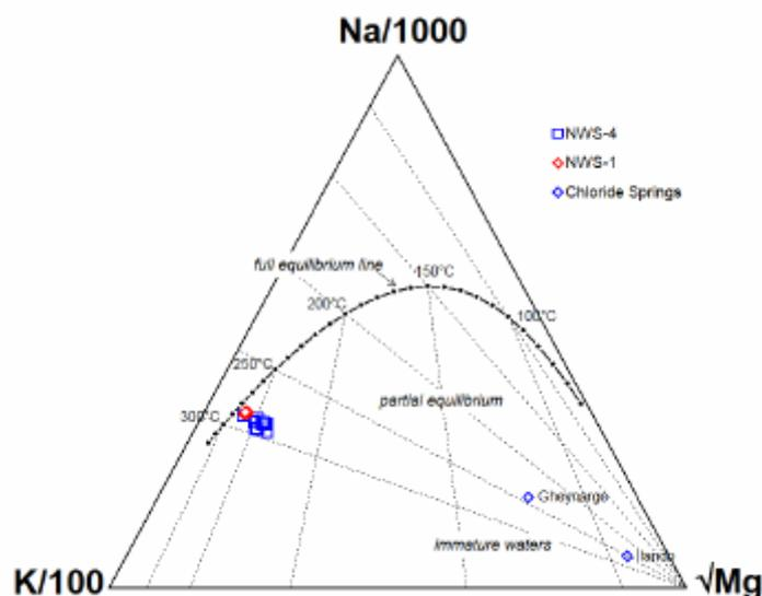
FIGURE 8: Giggenbach's geothermometer ternary diagram
