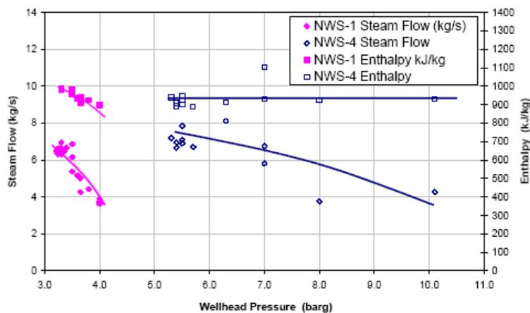
FIGURE 7: Output curves for wells NWS-1 and NWS-4
