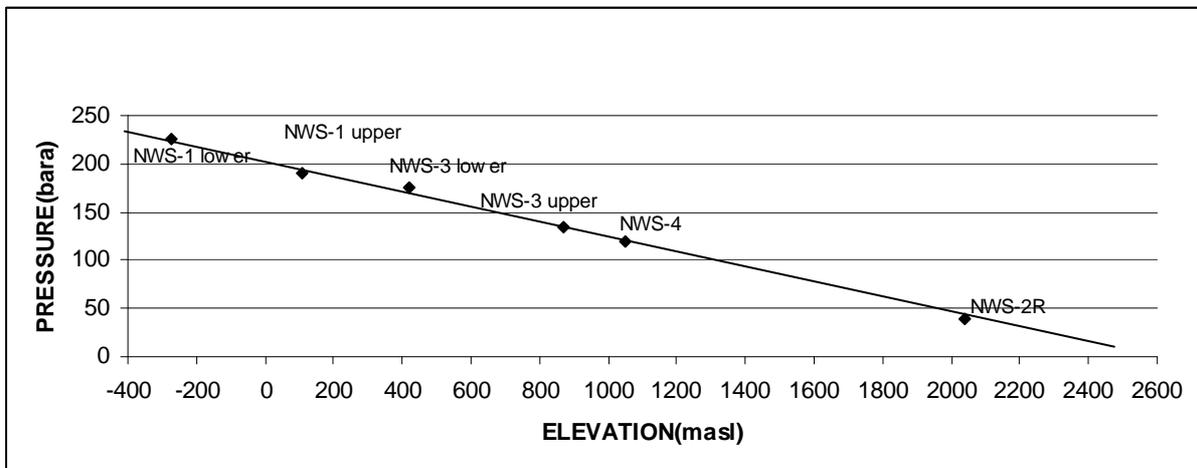
FIGURE 6: Pressure profile with depth (PCP plot)
