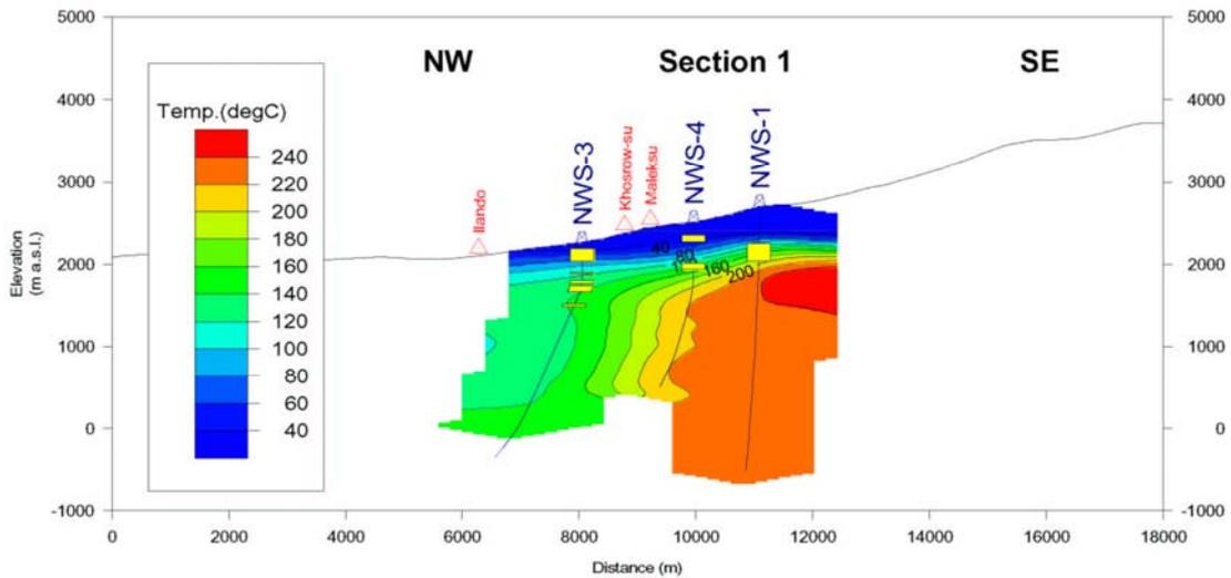
FIGURE 5: Sabalan vertical-section temperature contours
