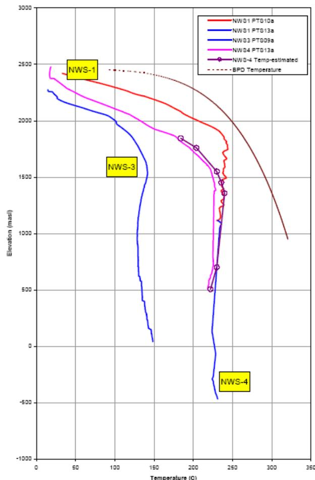
FIGURE 4: Estimated reservoir temperatures for the NW-Sabalan exploration wells
