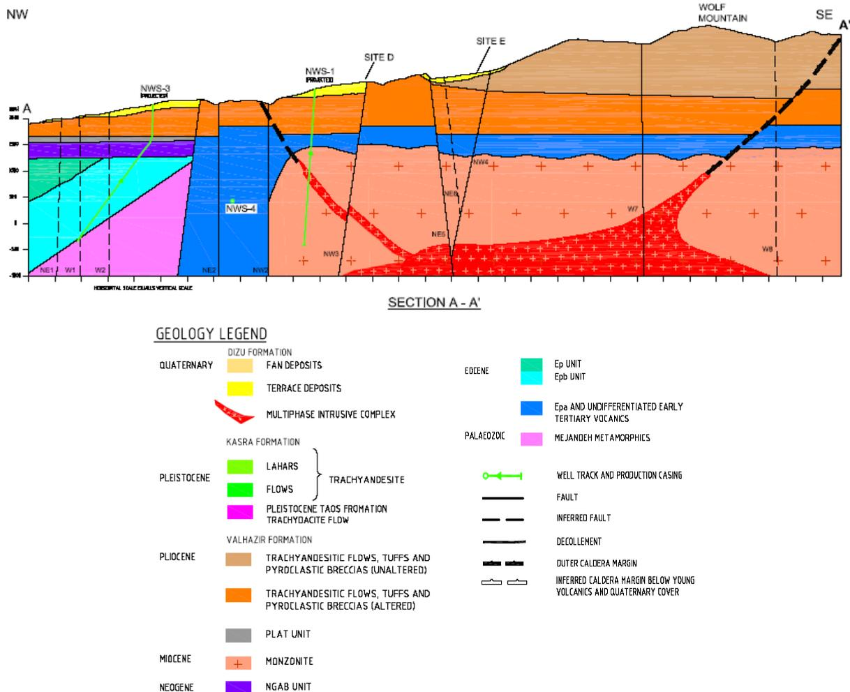
FIGURE 3: Geological cross section based on 3 wells exploration drilling
