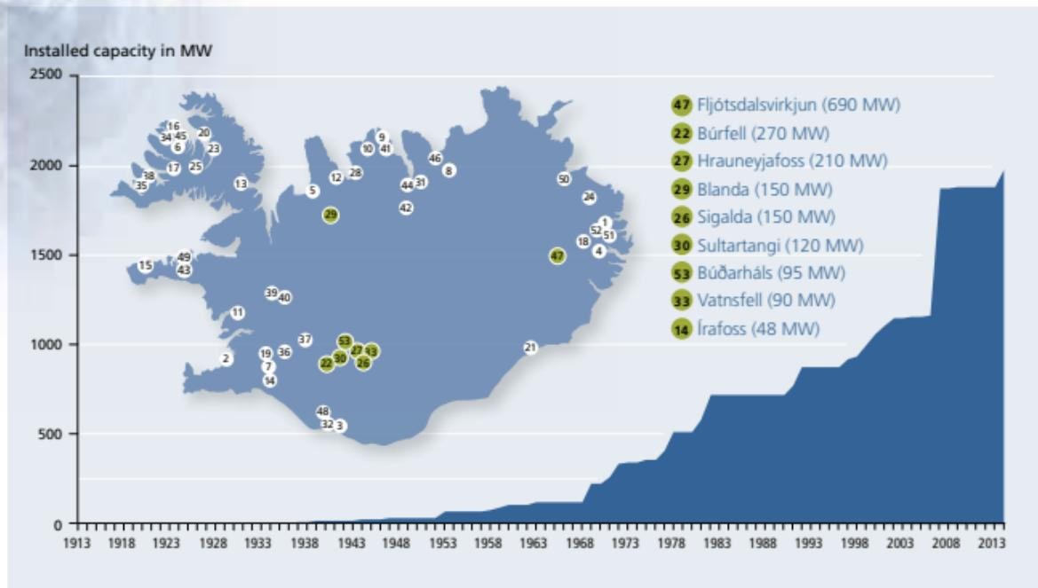
The numbered dots in the picture show the main hydro power plants in Iceland. The largest are specified (green dots).
