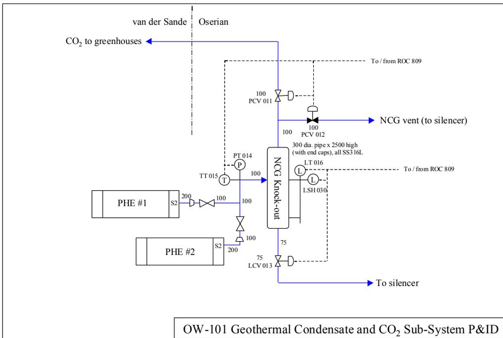
Figure 3: P&ID for Geothermal Condensate and CO<sub>2</sub> Sub-System.
