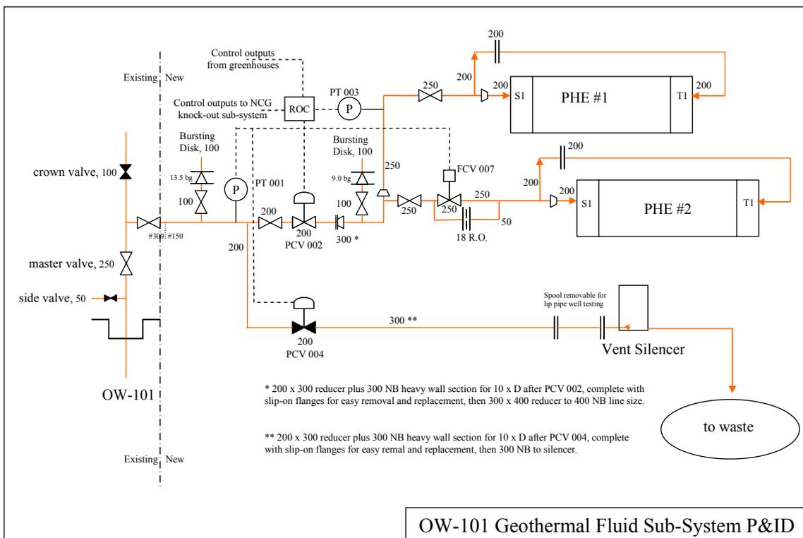
Figure 2: P&ID for Geothermal Fluid Sub-System.
