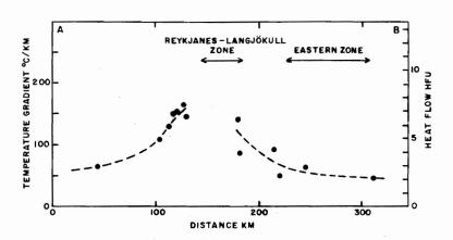
Fig. 2. Heat flow profile across the Reykjanes-Langjökull volcanic zone, which is a direct continuation of the crest zone of the Mid-Atlantic Ridge. The location of the profile is shown in Fig. 1. (From Palmason, 1973).
