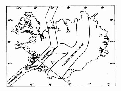
Fig. 1. Regional heat flow in Iceland. All the measurements are made in drillholes outside the active volcanic zones and outside known geothermal fields. Line A-B indicates the heat flow profile of Fig. 2. The two main active volcanic zones in Iceland are shown schematically. The arrows indicate the assumed directions of plate motion.
