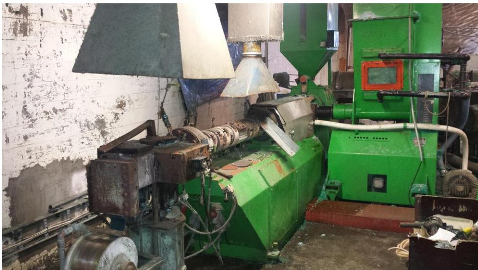
*Figure 6 - Plastic extruder unit*
