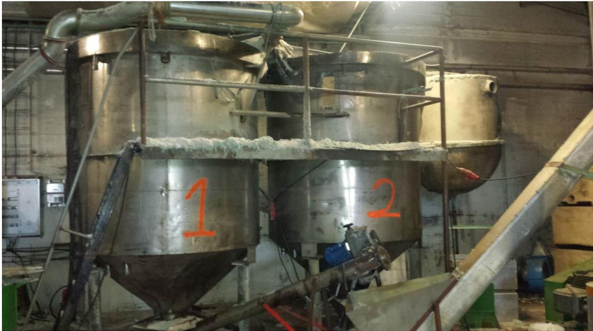
Figure 3 - Big size storage silo for shredded plastic
