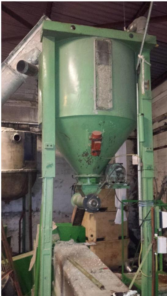
Figure 4 - Feeding system for plastic extruder unit
