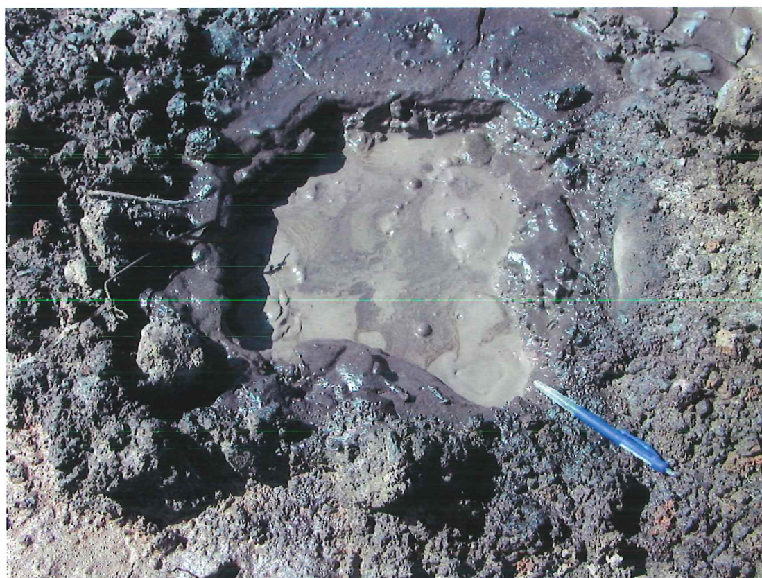
Photo 9. This is the boiling mud where the 4 m deep observation hole was drilled. Temperature measured 100°C so the bubbles are steam bubbles and not gas.
