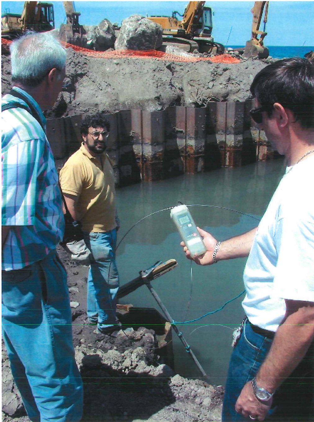
Photo 15. Temperature reading at location B in the bottom of the pit where the highest readings were obtained, 109°C at 5 m depth. When the picture is taken the reading is 104.5°C. Note the total length of the pipe that the thermocouple wire is strapped to is 6 m long.
