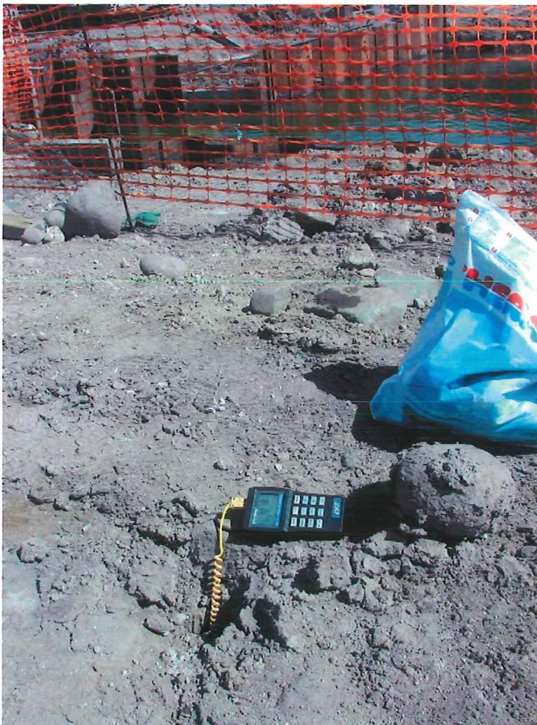
Photo 6. Shallow temperature reading in 19 m test well showing 101°C at 1 m depth.
