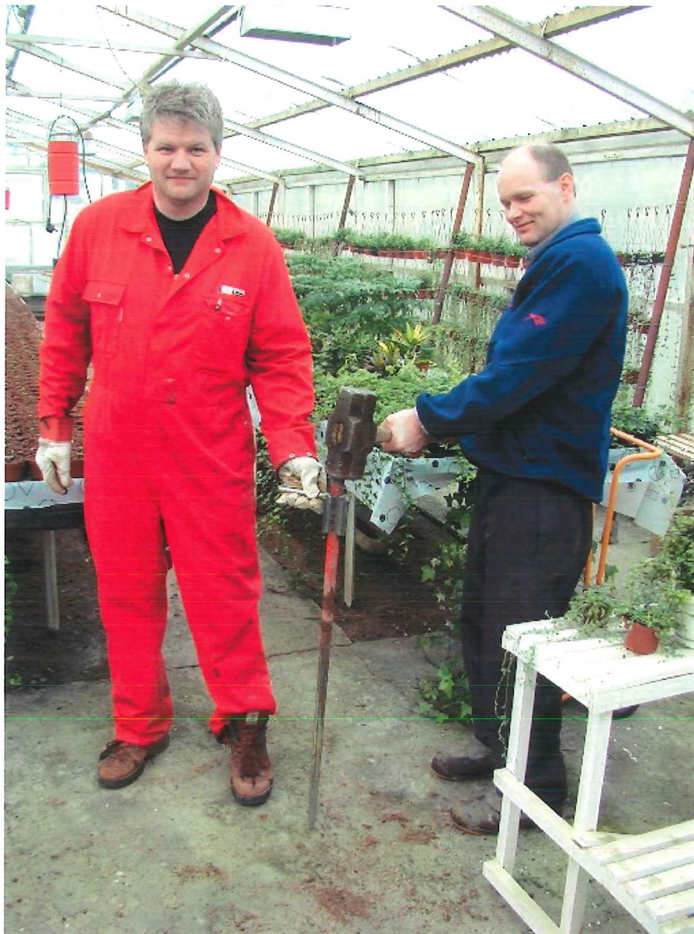
Photo 19. A steel chisel is first driven into the ground with a big sledgehammer to make a pilot hole for the temperature probe. The chisel is removed and the hole stays open. After temperature equilibration the temperature probe is lowered into the hole for the reading. Depth of reading in firm soil is usually 60 cm.
